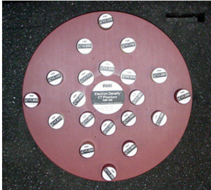
Figure 7 - Example of a phantom containing inserts of various densities. This type of phantom can be used in the determination of a CT number to relative electron density curve for an RTP system.
