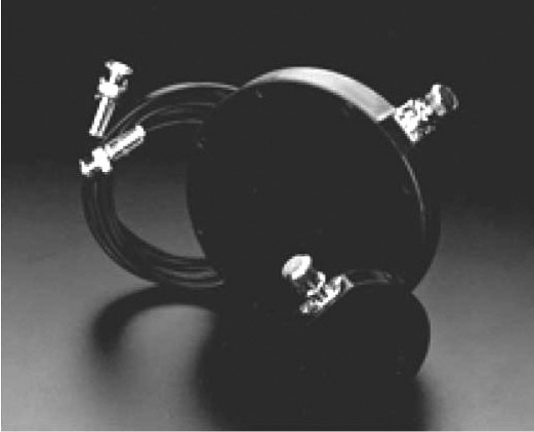
Figure 3 - A large volume (300 cm 3 ) ion chamber used in radiation survey of diagnostic equipment.
