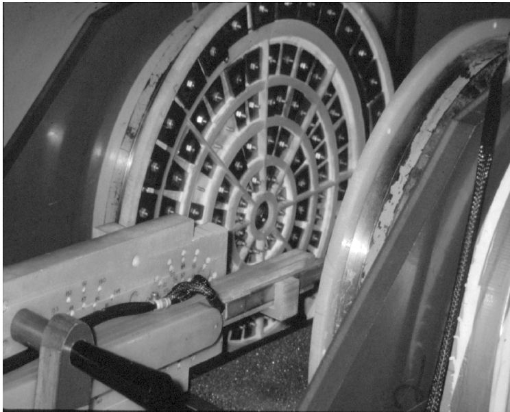
Figure 2. Close-up view of a pole piece and shimming tool for the 0.22T magnet. Optimizing the uniformity of the magnetic field requires manual adjustment of several hundred small shim elements to achieve uniformity (eventually) of about 40 ppm over a 10-cm-diameter spherical volume.
