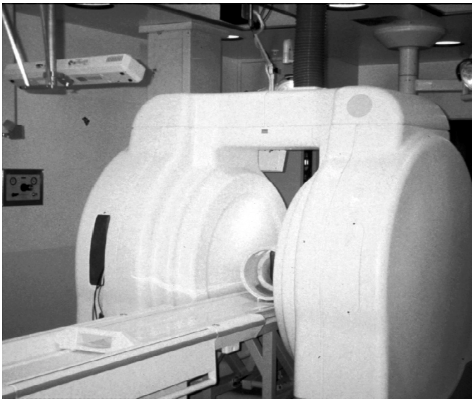
Figure 3. The IGMIT system at the Toronto Hospital has large vertical pole pieces with sufficient gap to allow the patient table to pass through the magnet. The overhead optical tracking camera and surgical lights can be seen.
